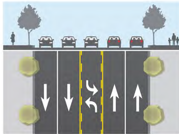
N ← ——— 10' TRAVEL LANE ——— 10' TRAVEL LANE ——— 10' DUAL LEFT TURN LANE ——— 10' TRAVEL LANE ——— 10' TRAVEL LANE ——— → S ————— 50' CURB-TO-CURB —————
